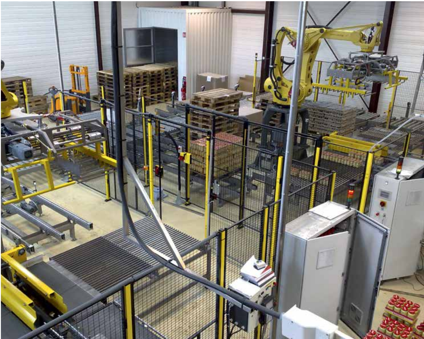
Axelent X-Guard®, height 2300 mm. The pictures show 25 metres of machine guard around a robot and pallets.
